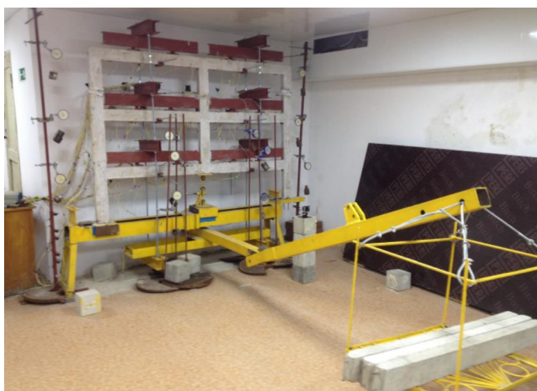
Figure 5 - General view of the test bench when testing frames N.V. Fedorova and Korenkov P.A. [8]
