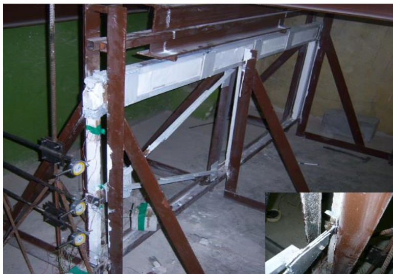
Figure 7 - General view of testing scale models of flat reinforced concrete frames of building frames [86]
